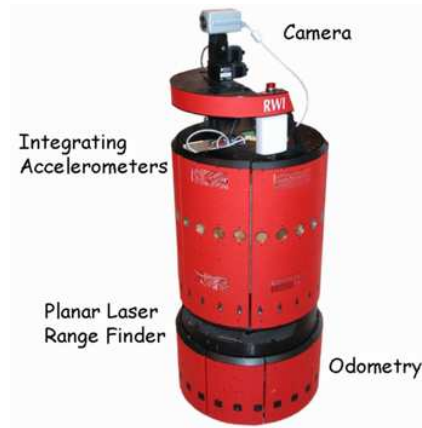
Figure 1: A B21r TM Mobile Robot from iRobot Corporation is an often used experimental robot platform. Autonomous systems may compute motion estimates with a large variety of different sensors. The goal of this paper is to study auto-calibration methods that find the rotation \Phi and the translation \Delta which relate the coordinate systems of different sensors, by considering data captured simultaneously from both sensors when the robot undergoes arbitrary motions in an unknown environment.
